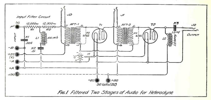
ties in the loud speaker and distortion in the final stages. To remedy this defect, the fixed stopping condenser (K3) of 1.0 mf. capacity is inserted in the plate circuit to interrupt the flow of continuous "B" battery current that ordinarily takes place through the coils of the loud speaker. This relieves the speaker diaphragm of the magnetic stress imposed upon it by the battery current and makes it more responsive as only the alternating audio currents can pass to the coils of the speaker.
