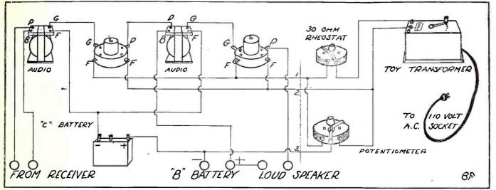
Complete wiring diagram of a two stage audio amplifier with filament current from the lamp socket. Ninety volts of "B" battery are used, with a potentiometer and  $4\frac{1}{2}$  volt "C" battery to eliminate the A. C. "hum."
