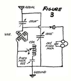
A diagram showing the connections of the crystal receiver which has done exceptionally good work for one of our Dial Twisters. The coil is a 40 turn inductance wound on a  $3\frac{1}{2}$  inch tube tapped every fifth turn. It is wound with No. 20 DSC wire.
