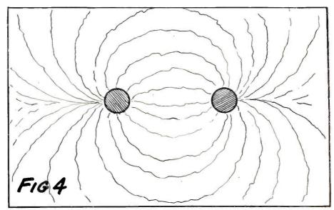
Electric field between oppositely charged conductors.
