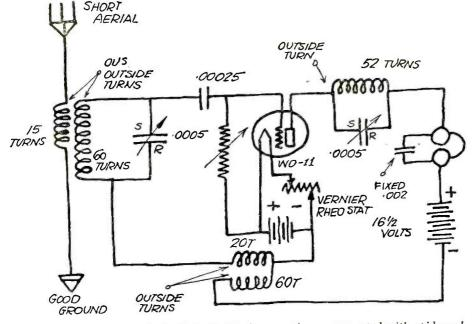
Figure 1. The diagram of the Baby Heterodyne receiver constructed with spiderweb coils as it was submitted to us by Mr Lueven of Los Angeles, California.
