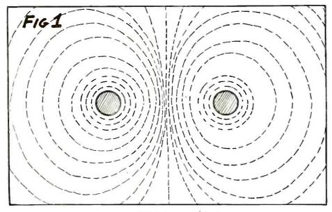
Magnetic field between conductors.
